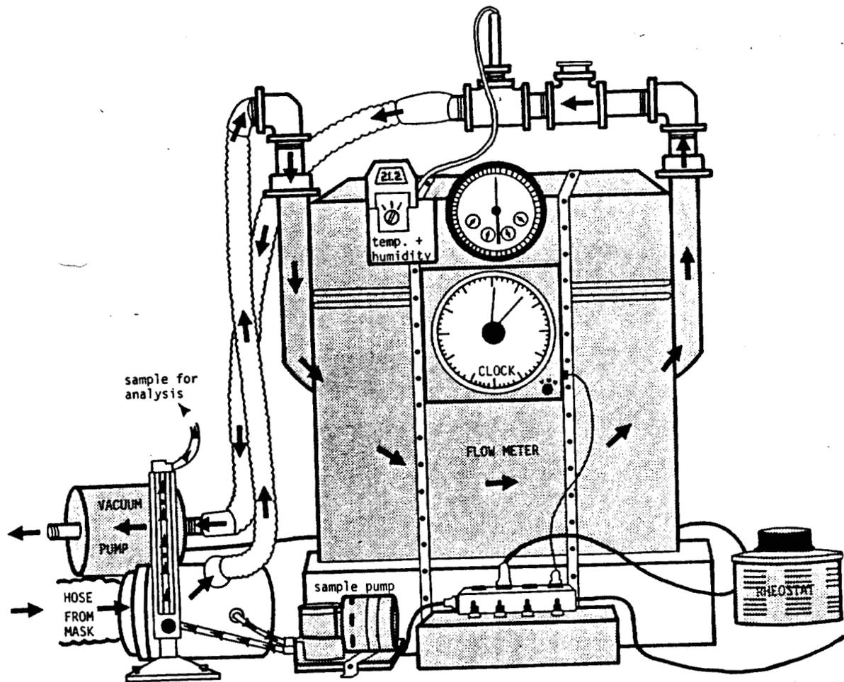
Figure 1. Modified open circuit indirect respiration calorimeter.
