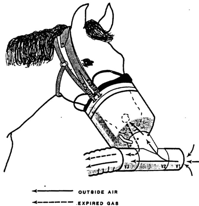
Figure 2. Face-mask used with respiration calorimeter.
